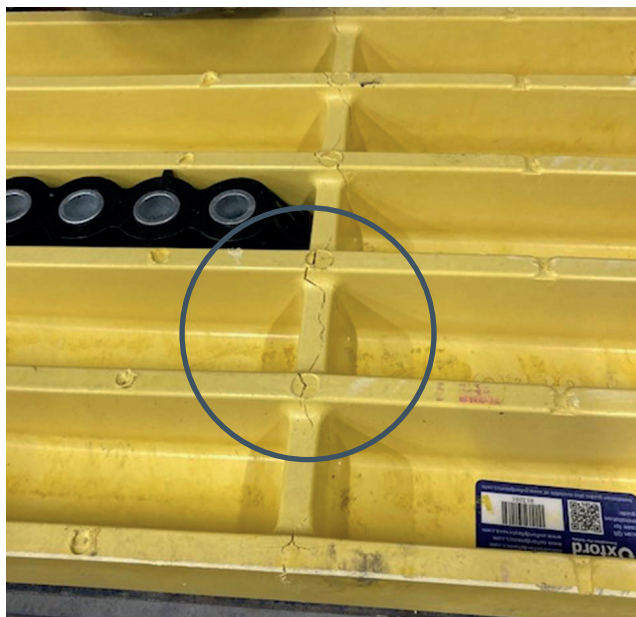
Crack along rib
